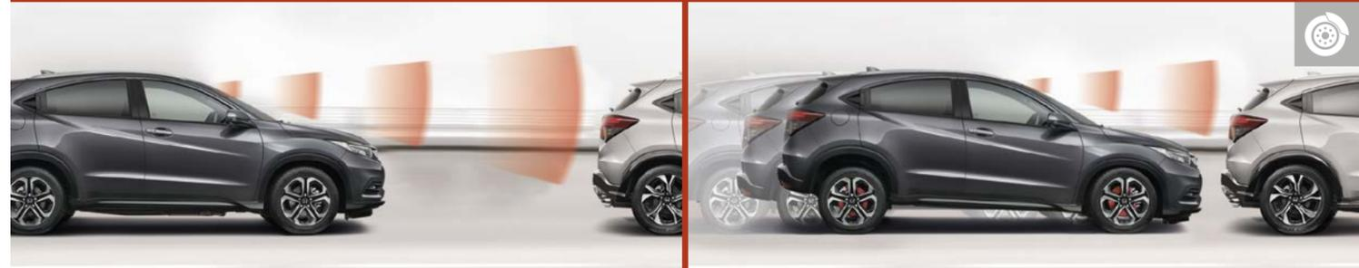
Acting as a second set of eyes, a laser sensor behind the rear view mirror monitors vehicles in front of you. In the event of a potential collision you're alerted with audible and visual warnings.
